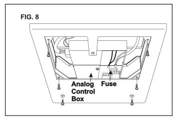
One test is to remove the fuse and do a continuity check. No continuity requires the fuse to be replaced. Another test can be done without removing the fuse. Use a DC voltmeter to check between ground and to each side of the fuse. If there is voltage on one side only, the fuse is bad and requires replacement.
