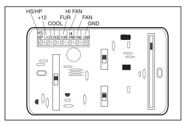
If any one of the volt readings is missing, check T-stat cable (B12) or analog control box (B14).
